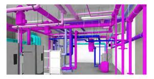
It includes parts that are necessary for coordination between disciplines with nearby or attached elements are modeled. This will include items such as supports and connections. The quantity, size, shape, location, and orientation of the element as designed can be measure from the model without referring to the non-modeled elements such as notes or call-outs.
